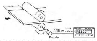
Note: The count will become incorrect if the prescale value is not prescale. Check the setting to be sure it is correct.
