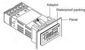
The H8GN's panel surface is water-resistive (conforming to NEMA 4X (indoors) and IP66). In order to prevent the internal circuit from water penetration through the space between the Counter and operating panel, attach a rubber packing (provided with the H8GN) between the Counter and operating panel and secure the rubber packing with the Flush-mounting Adaptor.
