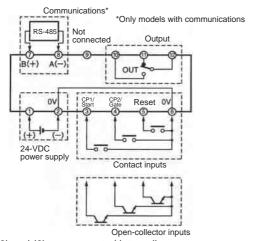
**Note:** (2) and (6) are connected internally. Do not use unused terminals as relay terminals.
