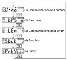
Align each communications setting with the settings on the personal computer or other communications device.
