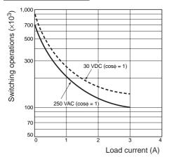
Reference: A maximum current of 0.15 A can be switched at  $125 \text{ VDC } (\cos\phi = 1)$  and a maximum current of 0.1 A can be switched if L/R is 7 ms. In both cases, a life of 100.000 operations can be expected. The minimum applicable load is 10 mA at 5 VDC (failure level: P).
